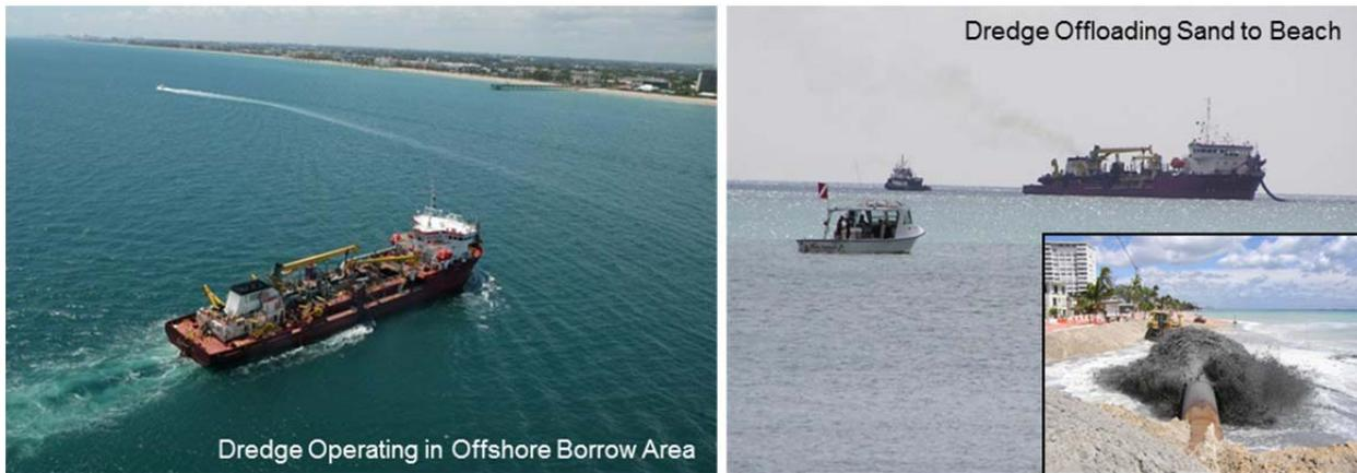
**Figure 6:** Typical construction operations associated with an offshore dredging for beach fill.
